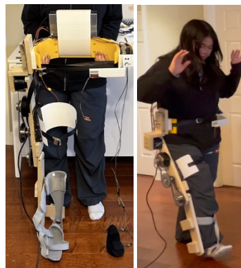
Figure 1: Front view of the built exoskeleton and the subject walking in the exoskeleton.
